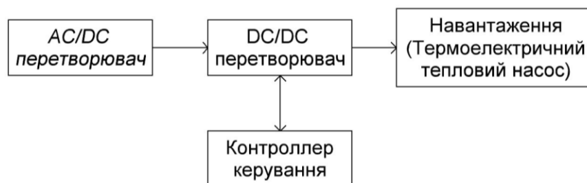
Figure 1 - Structural diagram of a powerful programmable current sources for use in control systems thermoelectric heat pumps
