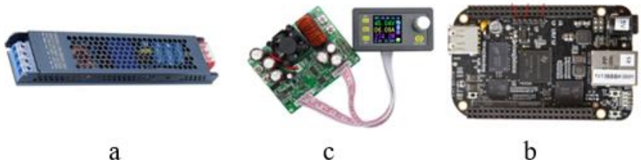
Figure 2 - a - power supply unit AC / DC CB -500 W -24 V; b - DC-DC converter DPS5020; single-board computer beaglebone black
