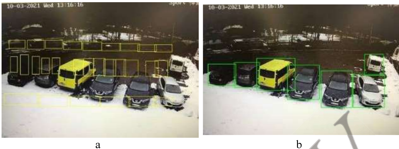
Fig. 3. Identified objects on the target image that correspond to the searched cars, found by: a – OpenCV + CNN, b – GCV API [13]
