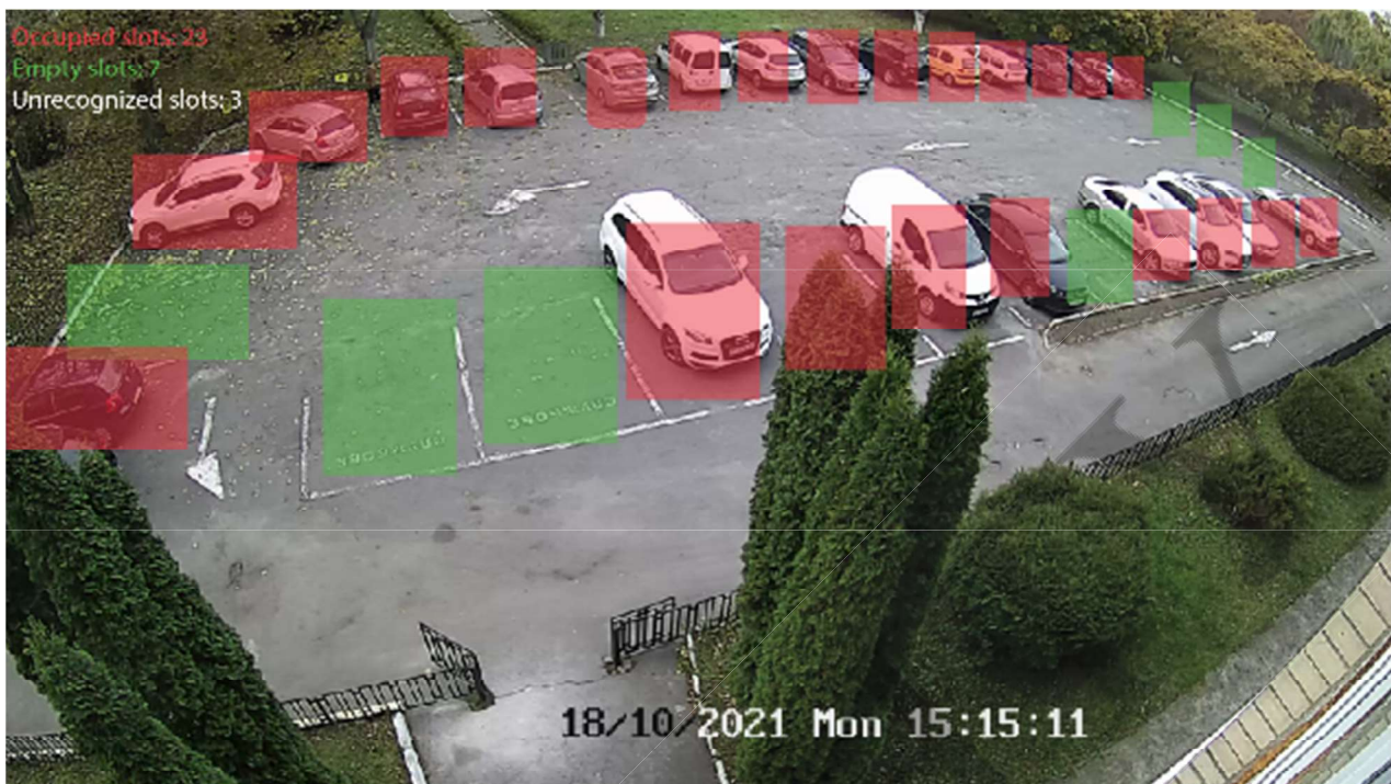
Fig. 9. The visualization sample of the parking lot: red color represents the occupied slots, green color – empty slots
