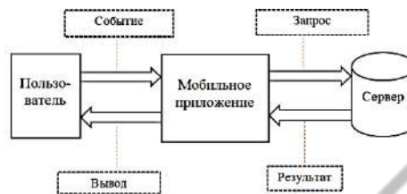
Figure 1 - Functional structure of the application
