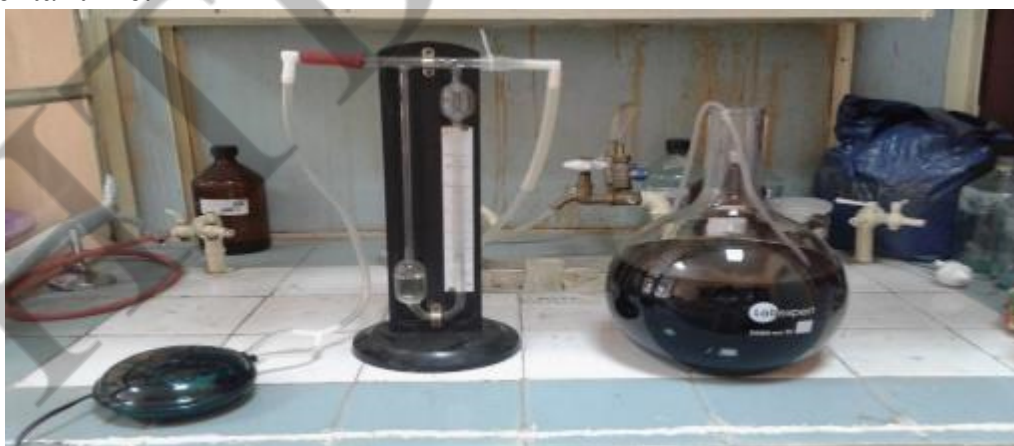
Ill. 3.1. Scheme of experimental plant for infiltrate aerobic purification.
