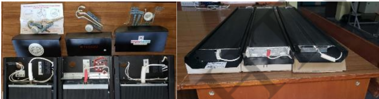
Fig. 3. Terminal connection, radiating plate connection and thermal insulation of the housing.
