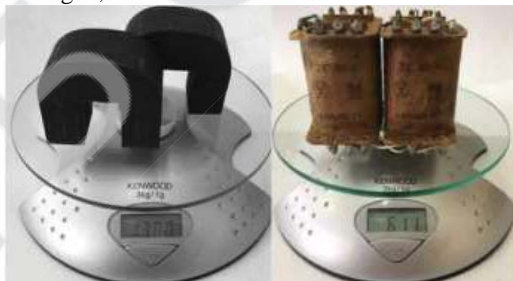
Fig. 6 - Elements of the active part of the transformer: a - magnetic circuit; b - winding system
