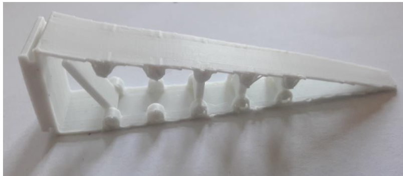
Fig.4.17. Type and location of failure of a finger made of Elastan material after fatigue testing
