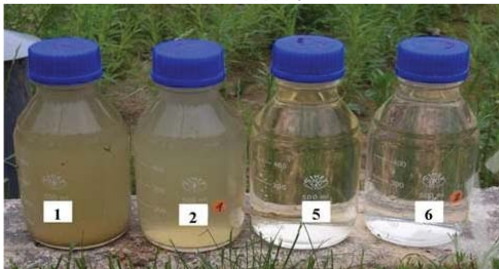
Wastewater from the VF-HF system: 1 – raw wastewater, 2 – after mechanical treatment, 5 – outflow from the VF bed, 6 - outflow from the HF bed [Jóźwiakowski 2012]
