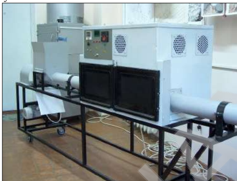
Fig. 1. Microwave device for thermal treatment of bulk materials
