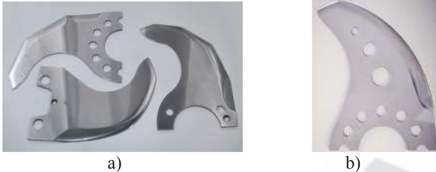
Fig. 1. Types of bowl cutter knives: a) –ordinary; b) –perforated.
