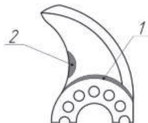
Fig. 2. Layout of stress concentration zones of the cutting knife: 1 – area near the mounting part of the knife, 2 – area on the back edge of the knife.
