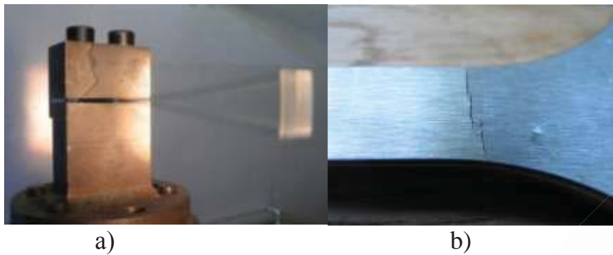
Fig. 3. Testing the sample for fatigue on the vibration testing machine VEDS-200A: a) – deformations of the sample during oscillations; b) – fatigue cracks on the sample.
