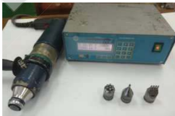
Fig. 5. Installation for surface hardening by high-frequency mechanical forging
