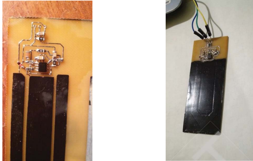
Fig. 13 - Sensor appearance before and after varnishing
