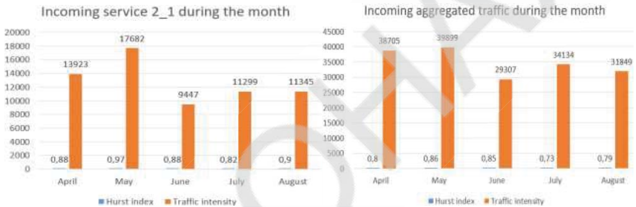
Fig. 5. Graphs of the relationship between the Hurst exponent and the intensity of incoming traffic for a period of months: a - service schedule 2_1, b - aggregated traffic schedule
