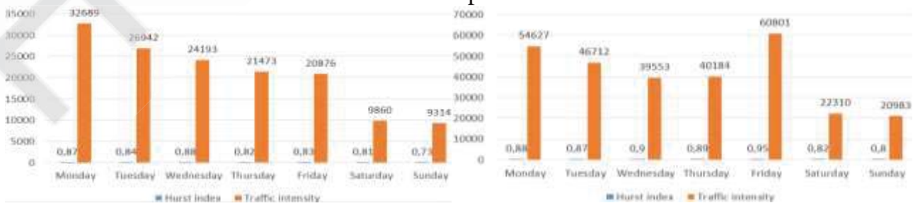
Fig. 3. Graphs of the relationship between the Hurst exponent and the intensity of incoming week traffic: a - graph of service 1_1, b - graph of aggregated traffic
