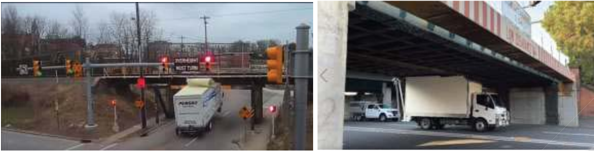
Picture 4. Failure of the driver to comply with the sign «Height limitation»
