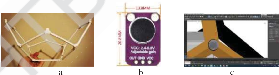
Fig. 6. Frame of a dodecahedron lamp (a) with the sound sensor (b) built in the vertex (c)
